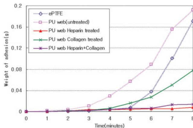
**Figure 9** Weight increase by thrombus adhesion to heparin- and collagen-treated specimens (PU = polyurethane). [Color figure can be viewed in the online issue, which is available at [www.interscience.wiley.com](http://www.interscience.wiley.com).]
