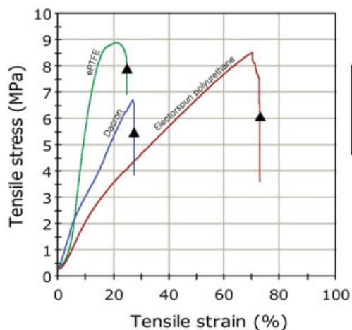
**Figure 7** Tensile properties of vascular prostheses. [Color figure can be viewed in the online issue, which is available at [www.interscience.wiley.com](http://www.interscience.wiley.com).]
