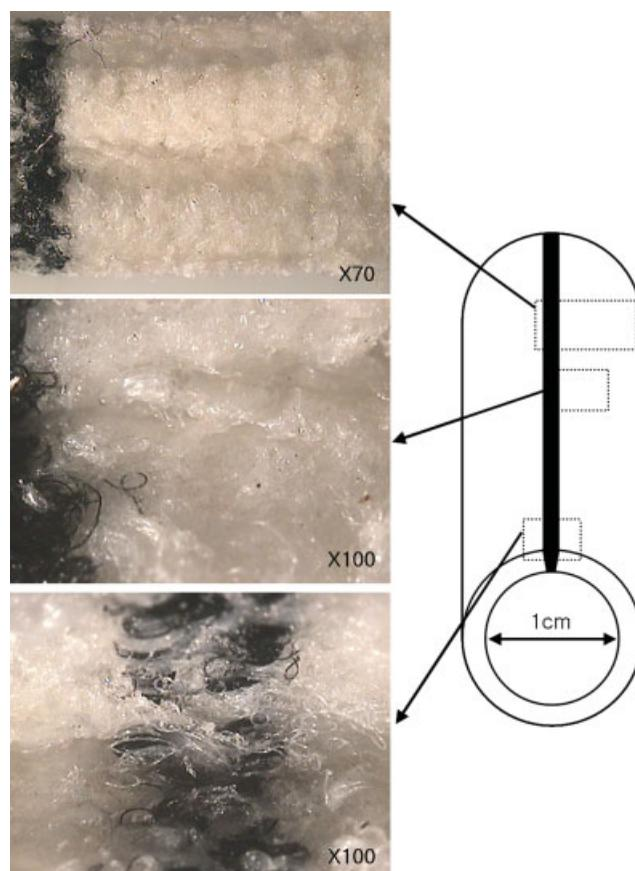
**Figure 4** Video microscopy pictures of ePTFE vascular prostheses. [Color figure can be viewed in the online issue, which is available at [www.interscience.wiley.com](http://www.interscience.wiley.com).]
