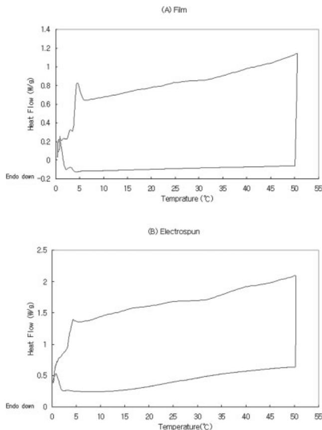
**Figure 2** DSC diagram of (A) a polyurethane film and (B) an electrospun web (maximum sensitivity = 0.2  $\mu$ W).
