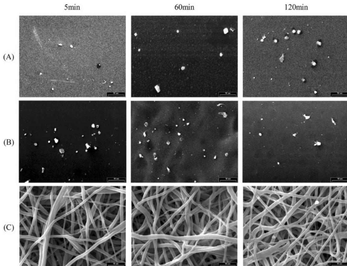
**Figure 6** Results of platelet adhesion testing: (A) glass, (B) polyurethane film, and (C) polyurethane web (SEM; magnification, 2000 $\times$ ).
