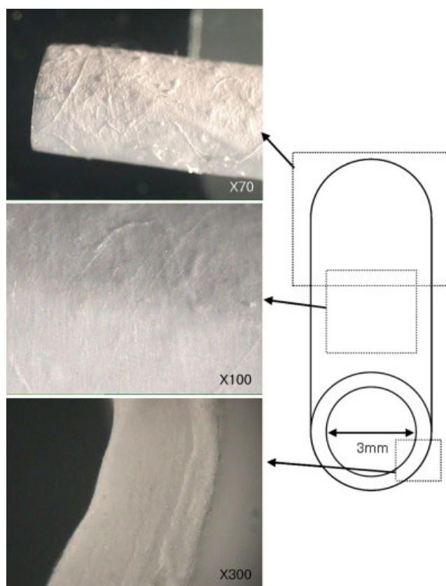
**Figure 5** Video microscopy pictures of electrospun polyurethane vascular prostheses. [Color figure can be viewed in the online issue, which is available at [www.interscience.wiley.com](http://www.interscience.wiley.com).]
