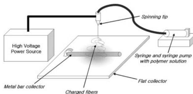
**Figure 1** Electrospinning scheme for making vascular prostheses.
