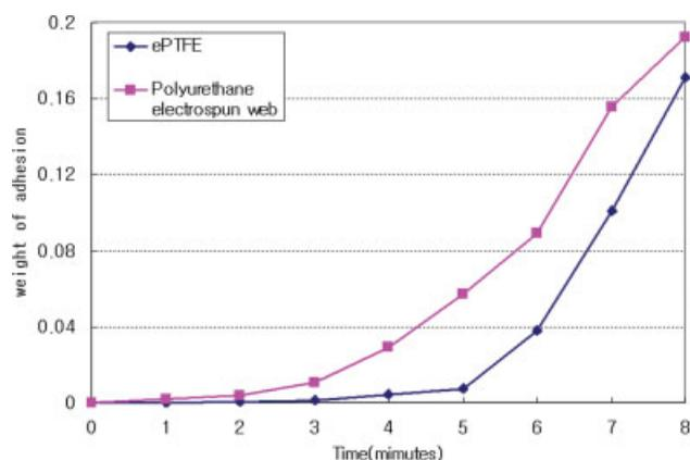
**Figure 8** Weight increase by thrombus adhesion to untreated specimens. [Color figure can be viewed in the online issue, which is available at [www.interscience.wiley.com](http://www.interscience.wiley.com).]
